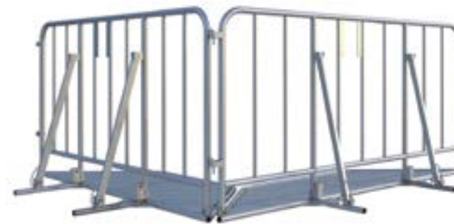
Police Barrier Collapsible Code: 02055240 Dimension: L:2187mm x H:1090mm x W:1004mm Frame dia: 33.7mm Weight: 48.5kg Finish: Post Galvanised
