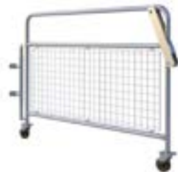
Police Barrier Gate HD (5ft) Code: 02055091 Dimension: L:1602mm x H:1106mm Frame: 33.7mm diameter Infill: 3.9mm dia Wire 50mm Aperture Weight: 22kg Finish: Post Galvanised
